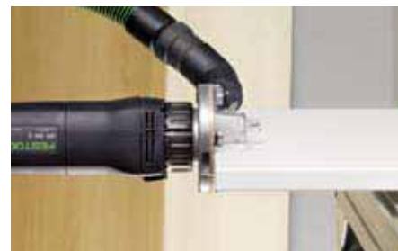
Rounding plastic or solid wood veneer.
