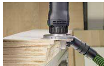
Chamfering plastic or solid wood veneer.
