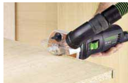
Flush trimming plastic or solid wood veneer.
