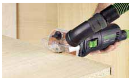
The use of an edge trimming cutter is recommended to make the edge banding or coatings and laminates perfectly flush with the workpiece.
