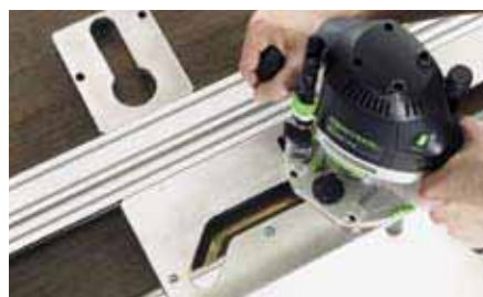
Quick manufacture of corner and panel joins using the worktop routing template.
