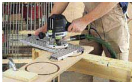
Producing round cut-outs with ease.
