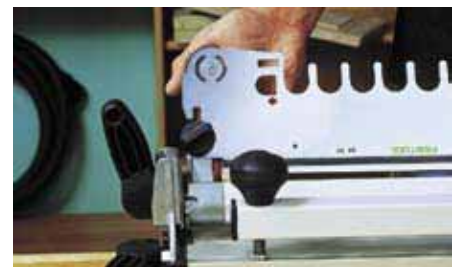
To be able to route several workpieces one after the other, the template is simply folded upwards. It does not need to be removed.
