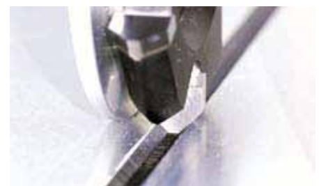
The feeler roller ensures precise routing depths. The router can only plunge into the material as far as the feeler roller allows.
