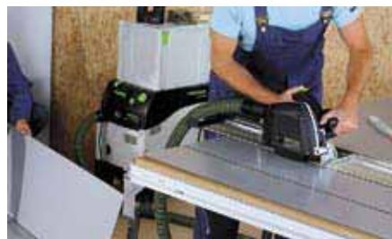
Efficient chip extraction with a 36 mm suction hose and a Festool mobile dust extractor.
