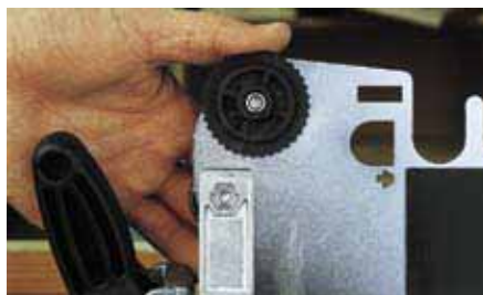
The memory eccentric disk and simple clamping system enable accurate, repeat positioning of workpieces and templates.
