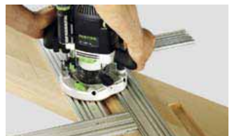
By using the MFS, even steps can be precisely routed in their stringers.
